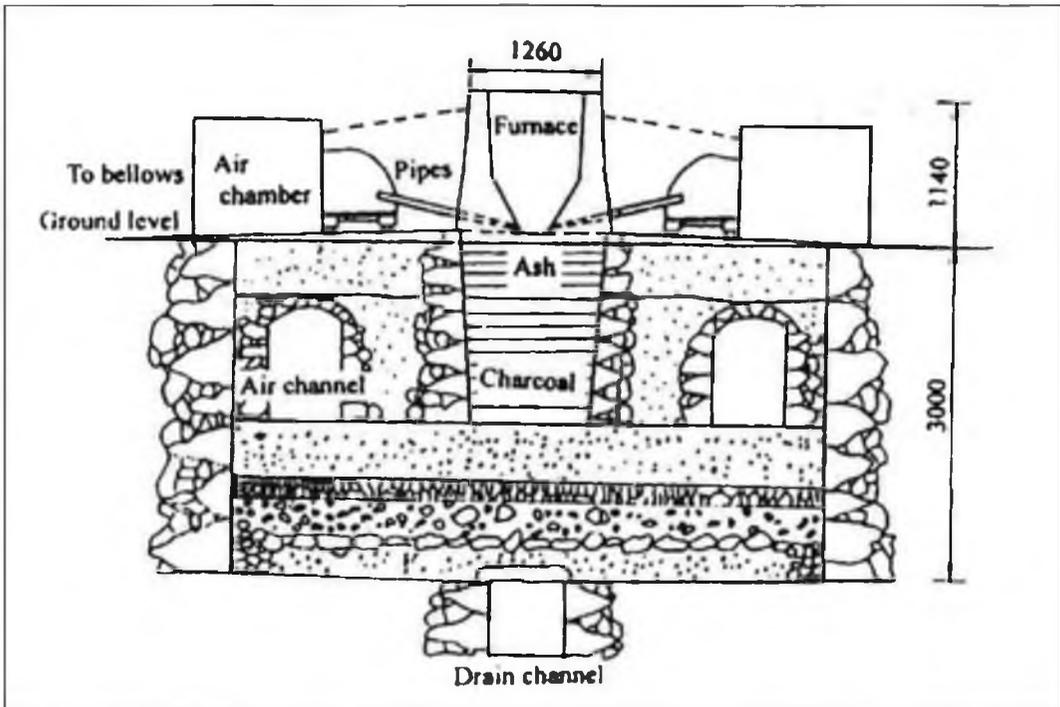
Figure 10 : Tatara ironmaking in Japan (Courtesy : T. Inoue)
