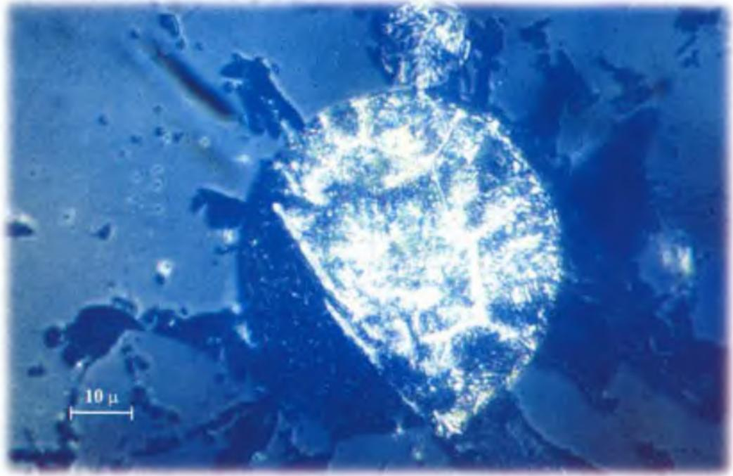
*Figure 54 : Microstructure of a cross section of crucible from Mel-siruvalur showing globule of steel*
