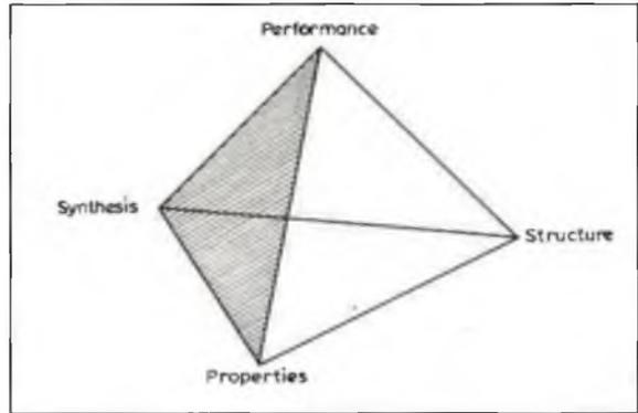
Figure 60 : Materials tetrahedron indicating relation among structure, properties, processing and performance
