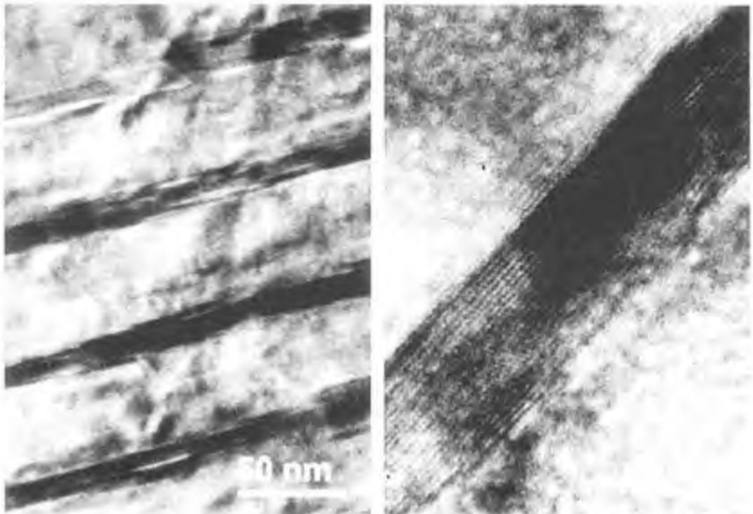
*Figure 62 : Detection of nanowires in Damascus steel. High resolution transmission electron microscopic images reveal nanowires of cementite several hundred nanometers in length (Courtesy : Werner Kochmann)*
