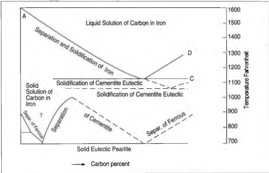
Figure 12 : Iron-carbon (Fe-C) diagram (first phase diagram of any alloy to be established, done by Roberts-Austen in 1898 after whom austenite came to be named)
