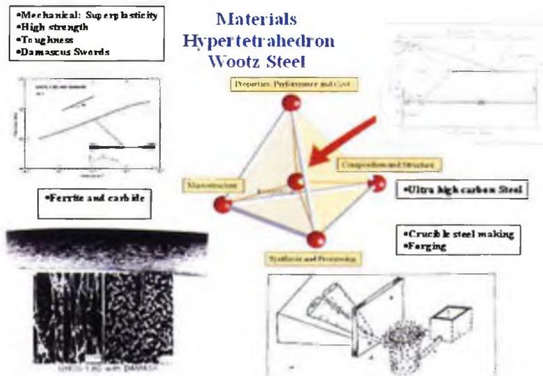
Figure 61 : Materials hypertetrahedron for Wootz steel indicating the materials relationships
