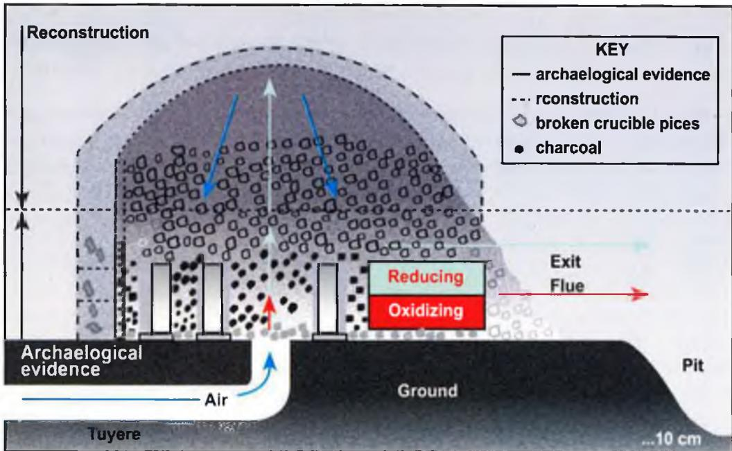
Figure 58 : Ironmaking furnace uncovered in Merv (Courtesy : Ann Feuerbach)
