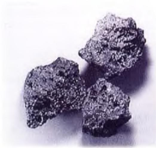
*Figure 11 : Tama hagana - Special Japanese iron made by the Tataru process (Courtesy : T. Inoue)*
