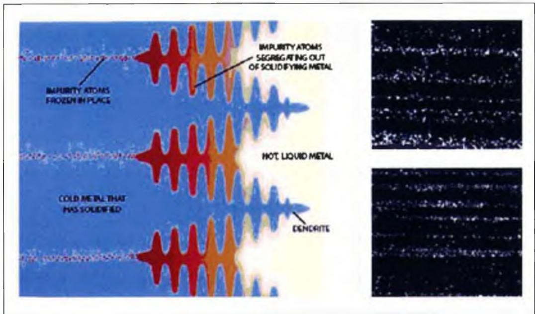
Figure 39 : Banding in vanadium containing steels. The dendrites form on solidification and vanadium segregates in the interdendritic space. During subsequent cooling and heating cycles this forms the basis for carbide formation and the ultimate pattern (Courtesy : J. D. Verhoeven)
