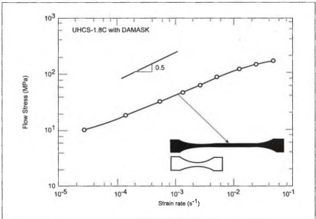
Figure 37 : Superplastic flow in ultra-high carbon steel (Courtesy : O. D. Sherby and J. D. Wadsworth)
