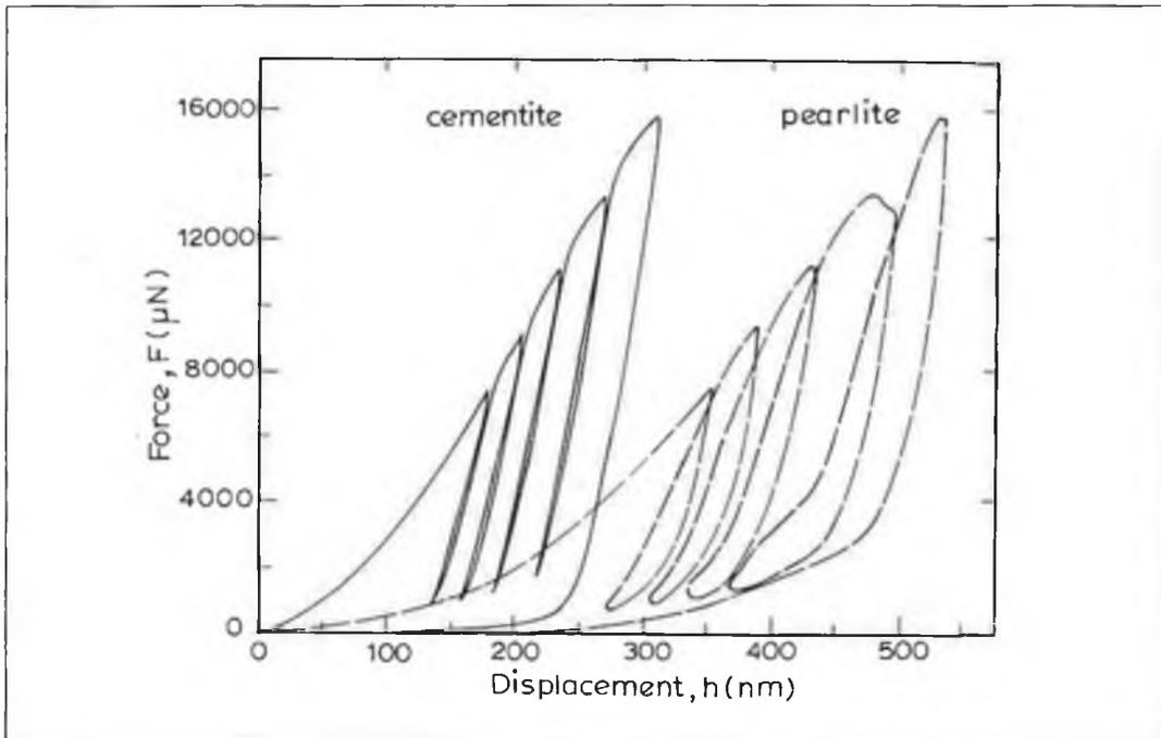
Figure 63 : Nanoindentation of cementite and pearlite. Force-displacement curves indicate a pronounced hysteresis in pearlite and none in cementite (Courtesy : Werner Kochmann)
