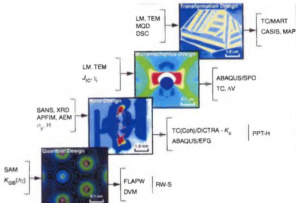
Figure 64 : Multiscale modelling is used to link different length and time scales. Both computation and experimental techniques are now available to go from the atomic- through nano-, meso-, micro- to macro-levels (Courtesy : G. B. Olson)
