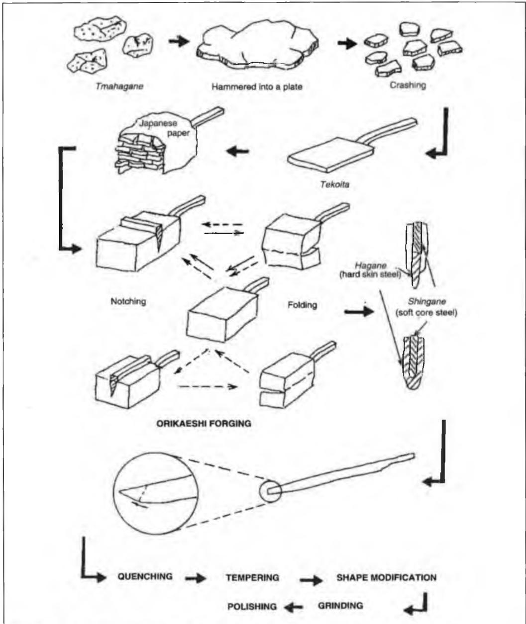
Figure 43 : Multiple steps involved in the making of a Japanese sword (Courtesy : T. Inoue)
