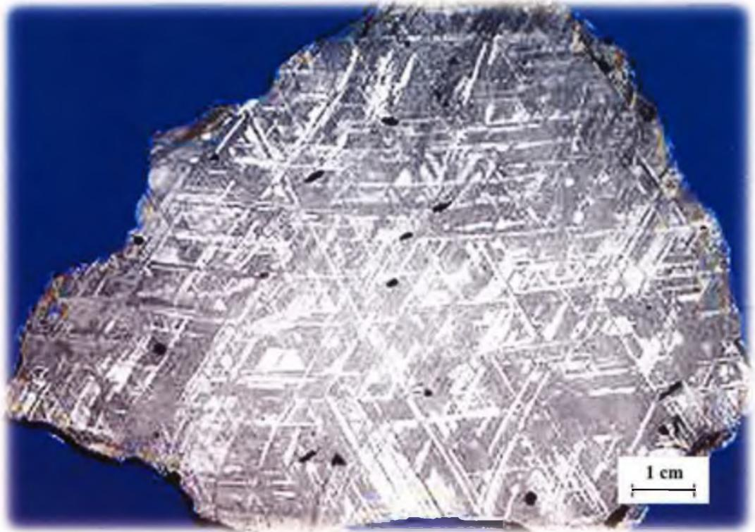
*Figure 7 : Widmanstätten pattern in meteoritic iron. Note the beautiful geometry of the pattern and the scale visible to the naked eye*
