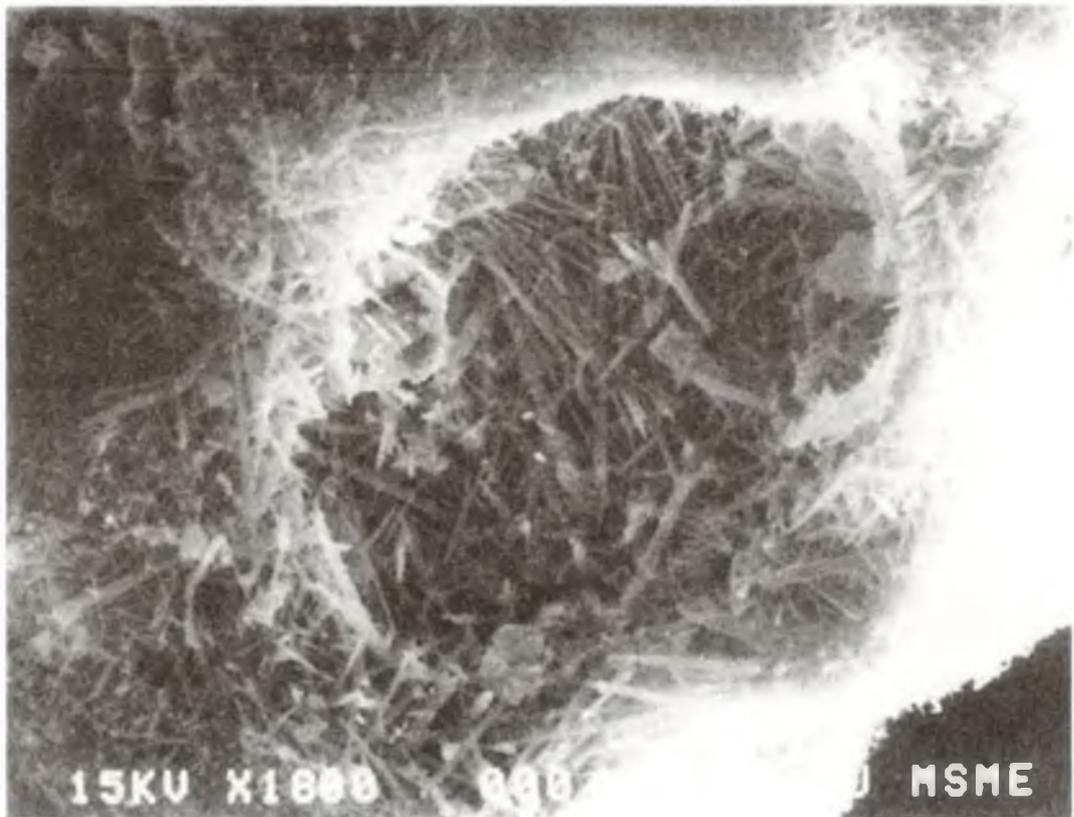
Figure 56 : Scanning electron micrograph of mullite network in the refractory of the crucible
