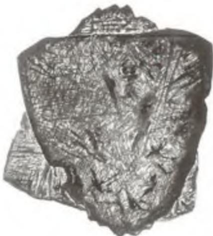
Figure 30 : Sketch of etched structure of wootz ingot revealing dendrites
