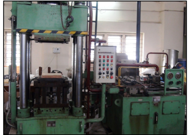
Figure 3: A 300 Ton hydraulic with a chemically treated jute felt on the platen for compression moulding.
