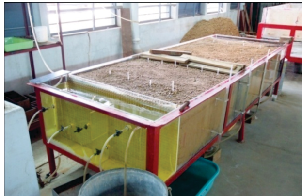
Fig. 1: Pilot scale reactor for bio barrier
