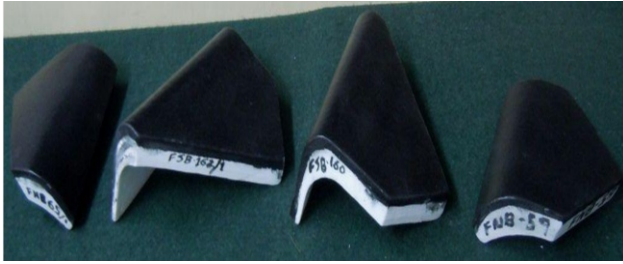
Silica tiles of different contours for Windward Regions of RLV-TD
