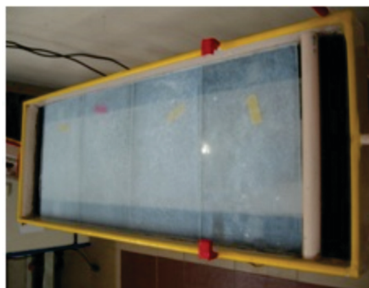
Fig. 4. Thin film continuous photo reactor for disinfection
