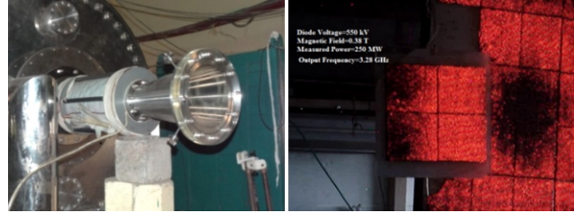
Fig. 4 Backward wave oscillator & output HPM on Neon bulb arrays in \text{TM}_{01} mode
