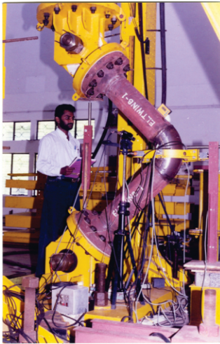
Figure 2: Photograph of elbow test set-up validation of the proposed improvements. The major analytical works are as follows:
