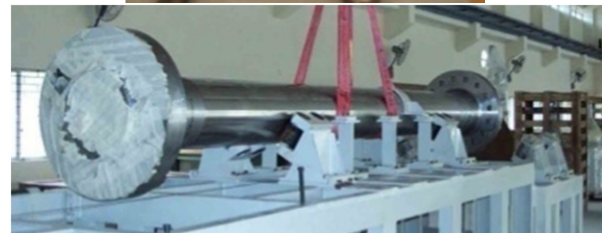
Fig. 13 - 15-5 PH forging & machined tube C. Combustion driver
