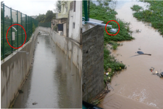
Figure 8: Water level sensor installed in a storm water drain and in a lake – Bangalore City case study
