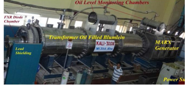
Fig. 3: Photograph of KALI-30GW system( 1\text{MV}, 30\text{kA}, 80\text{ns} )
