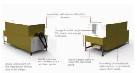
Deseeding efficiency < 50 % Capacity: 50-60 kg/h Power requirement: 0.4 units/h
