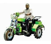
It has high turning radius hence difficult to maneuver, more loss of time in turning hence less field efficiency; farmers didn't accept the design.
