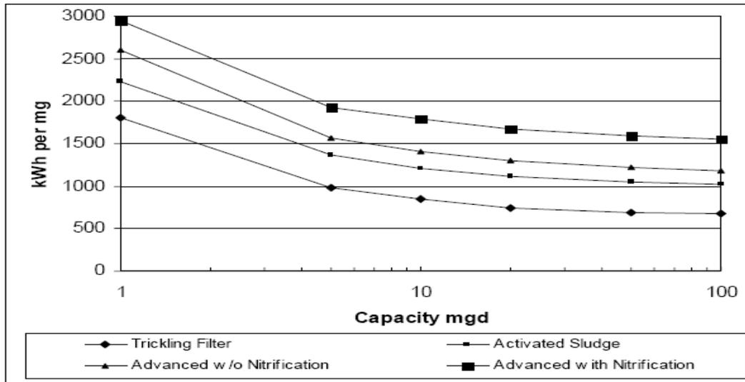
**Figure 6.7: Variations in Unit Electricity Consumption with Size for Representative Wastewater Treatment Processes [20]**
