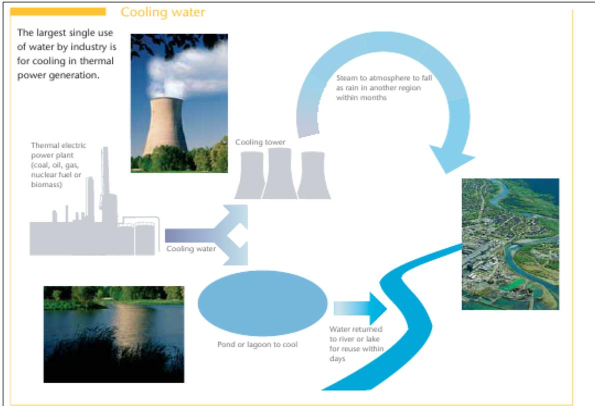
**Figure 6.9 : Water Used For Cooling in Thermal Power Generation [2]**
