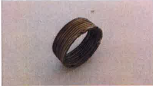
A ring made of pure titanium is 15 millimeters in diameter and five millimeters tall.
