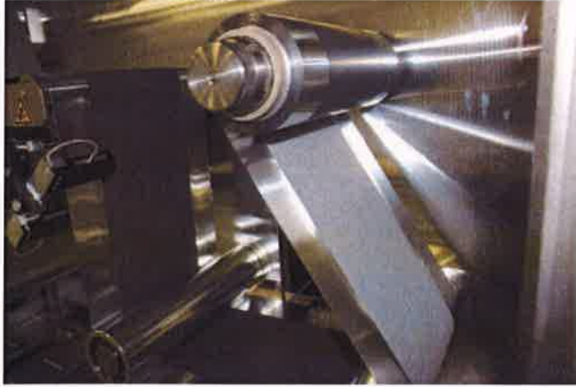
Production of the bipolar electrode on a pilot scale.
