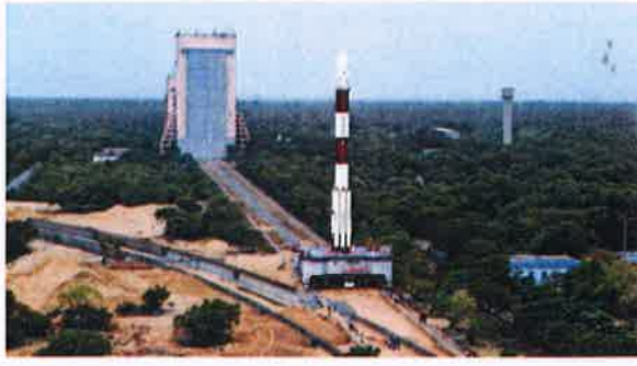
Panoramic View of Fully integrated PSLV-C34 with all the 20 Spacecrafts being moved to second launch pad (SLP).
