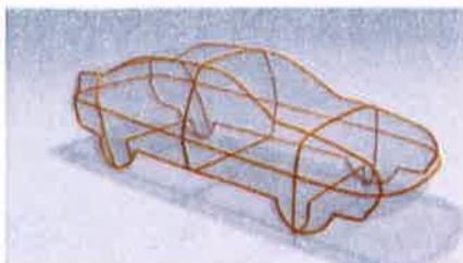
*Algorithm corrects connection points of objects fabricated by wire bending machine to optimize stability. Adaptions of design and structure computed. Potential range of application in Rapid Prototyping.*
