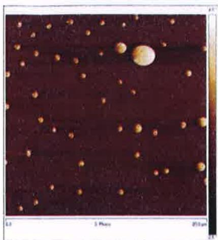
*Detail of the phase separation in the copolymer: when the siloxane (areas where yellow predominates) migrates to the surface, it generates greater roughness, and due to its hydrophobic characteristics, prevents the adhesion of organisms.*
