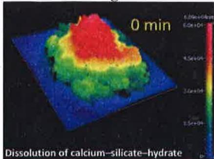
*This is a visualization of the dissolution of a C-S-H grain following its repetitive contact with an aqueous solvent. These visualizations which were enabled using vertical scanning interferometry (VSI) provide access to the surface topography at nanoscale resolution.*
