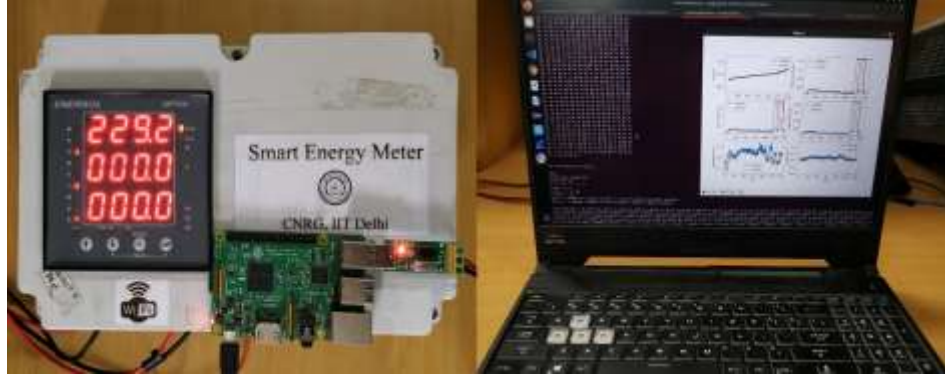
Figure 1: Deployed DLMS server (data-smart meter) and DLMS client.
