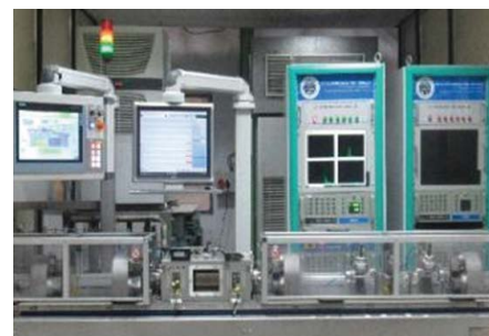
Fig-10: Probe rotating UT system
