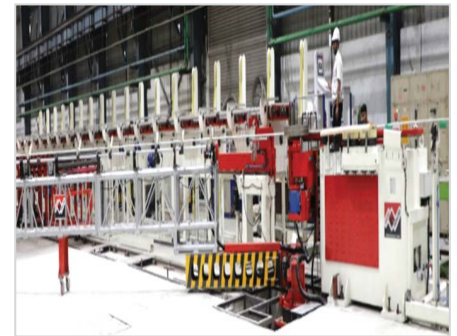
Fig-4: CNC U Bending machine with handling system
