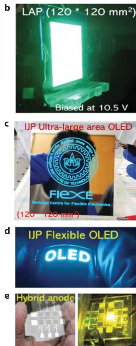
Figure 3. a) Inkjet-printed phosphorescent OLED using PO-01/CBP emitter on a flexible ITO substrate. The device, with dimensions of 5 × 10 mm 2 , demonstrates bright emission on bending, highlighting its potential for wearable displays. b) Large-area (120 × 120 mm 2 ) inkjet-printed OLED employing a TADF (thermally activated delayed fluorescence) emitter, operated at a bias of 10.5 V. c) Ultra-large-area OLED fabricated on an inkjet-printed dielectric template using SU-8 epoxy to pattern ITO electrodes. The printed pattern showcases institutional branding and precision. d) Flexible OLED device with inkjet-printed emissive text, illustrating the ability to integrate graphics and displays on flexible surfaces. e) Hybrid anode-based OLED. Left: Fabricated on a 50 × 50 mm 2 substrate using HC PEDOT:PSS as the transparent electrode, with inkjet-printed silver defining 4 × 4 mm 2 pixel areas for uniform charge distribution. Right: Illuminated OLED demonstrating successful operation without conventional ITO, enabling scalable, ITO-free display architectures.
