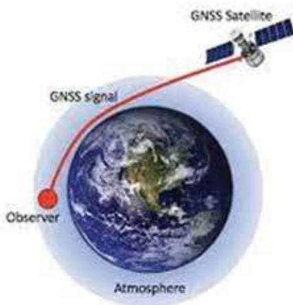
Fig 5. GNSS Radio occultation method
