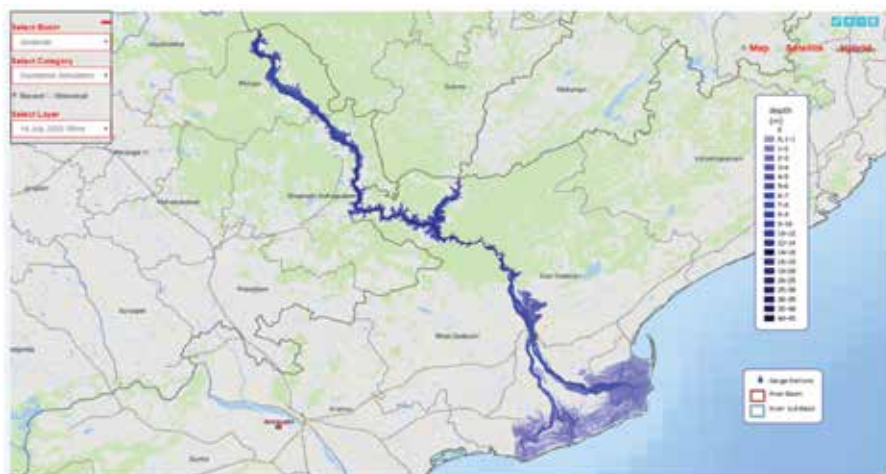
Figure 6. Simulated flood inundation at 08:00 hours on 14 July, for Godawari river
