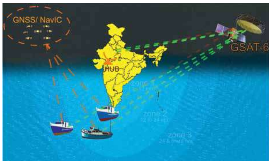
Figure 3. Fishing vessels monitoring system using S-band in GSAT-6 satellite
