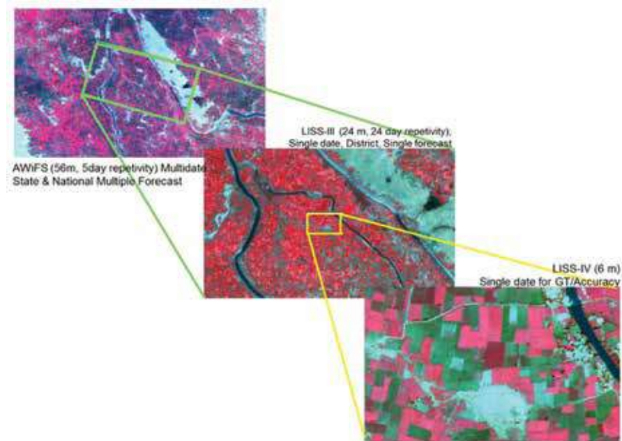
Fig 2 Crop monitoring using Remote Sensing Data from different sensors
